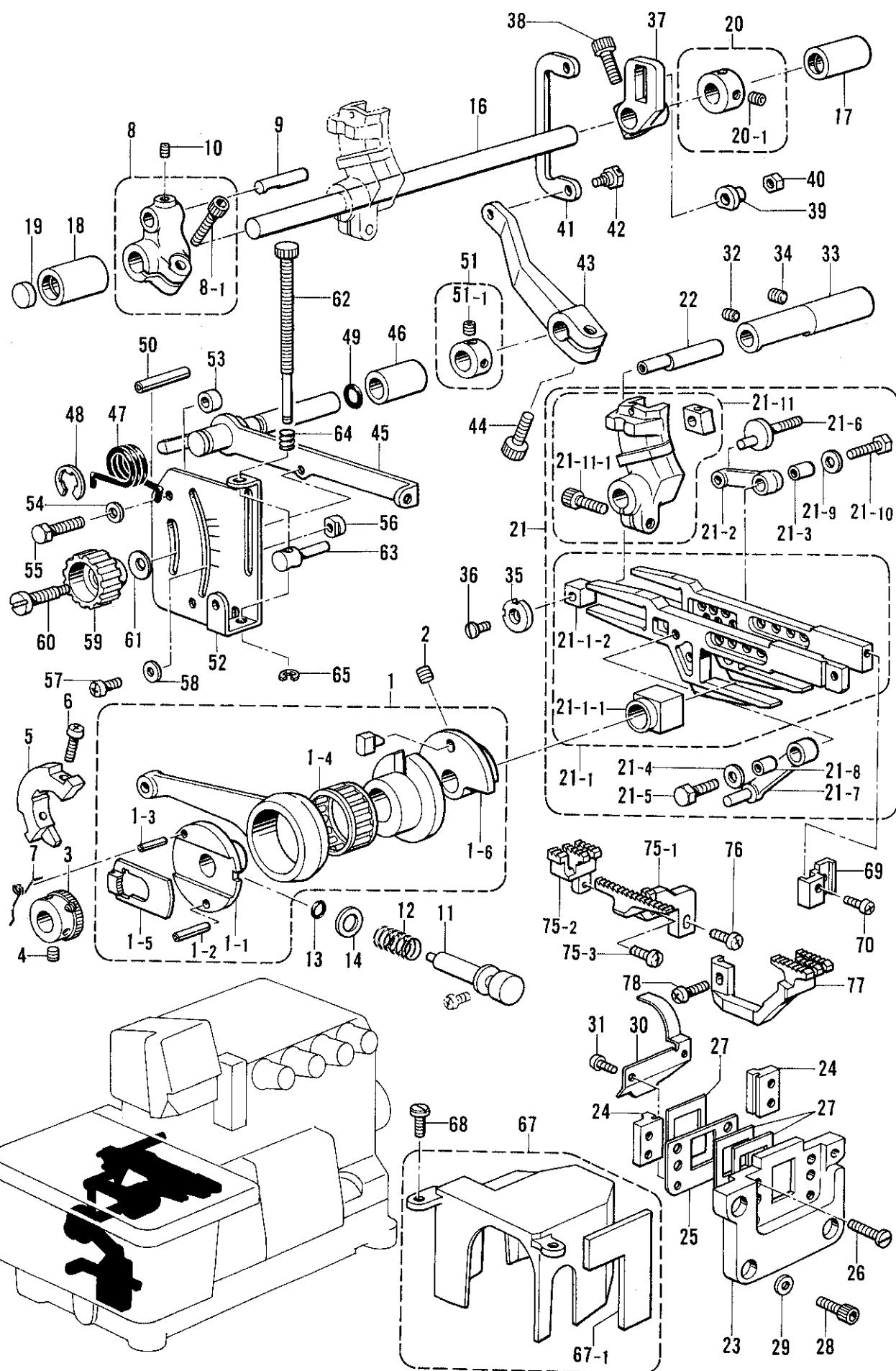
E. 送リ関係/Feed mechanism/Transportvorrichtung/
