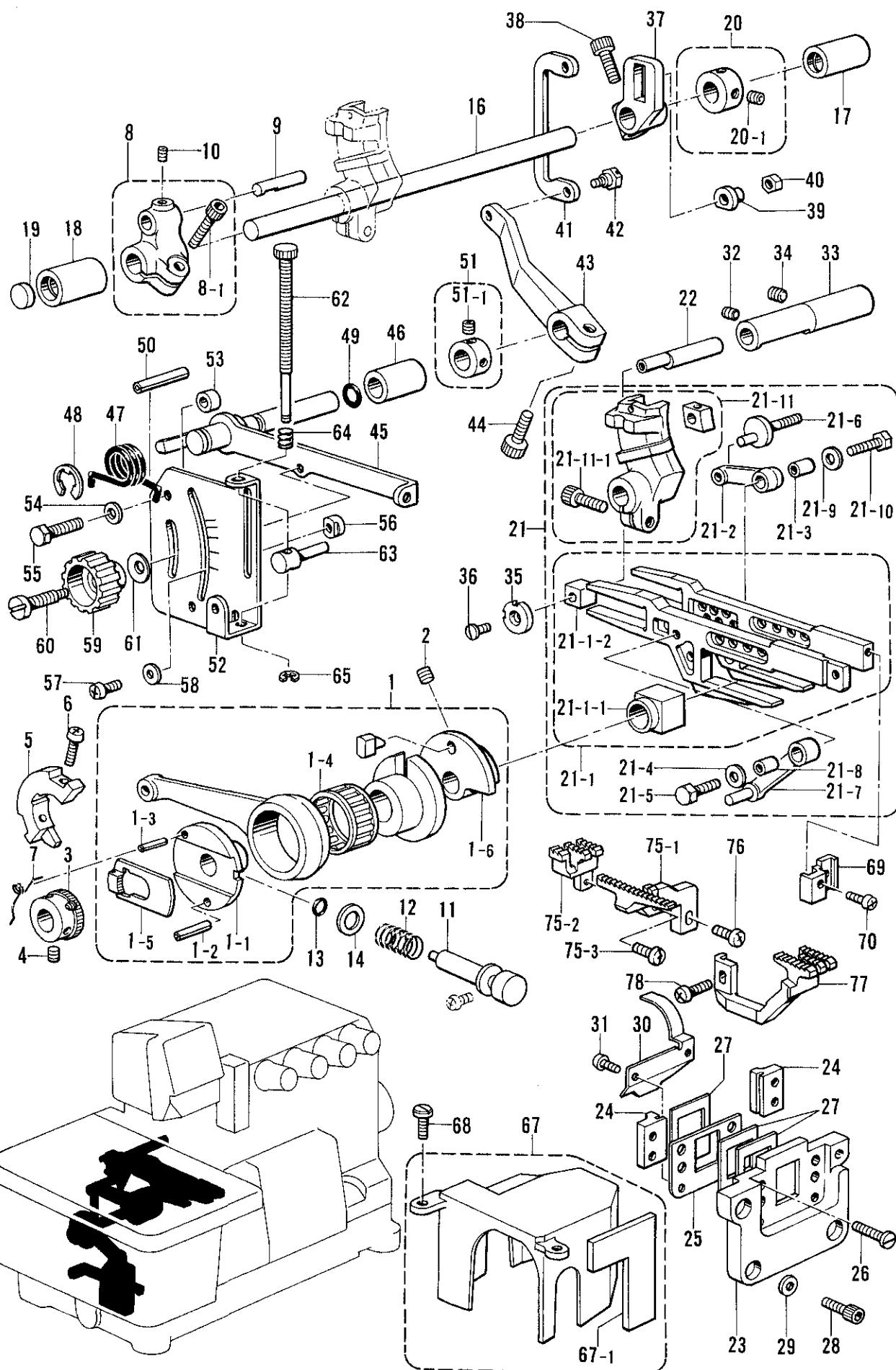
E. 送り関係/Feed mechanism/Transportvorrichtung/
